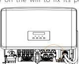
c) Use the inner hexagonal wrench to tighten the inner hexagonal screw on the right side of the inverter.
