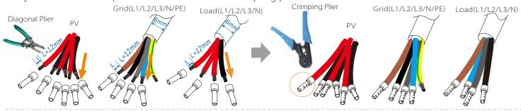
b) Grid (PE) strip the grounding cable, remove the 13 mm insulation layer from the end of the wire. Insert the stripped cable into the R type terminal, and then clamp it.
