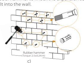
inner hexagonal wrench to screw the tapping screw until the expansion bolt "bang" is heard.
