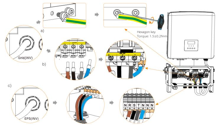
2) PV (PV1+/PV1-/PV2+/PV2-) /Grid (L1/L2/L3/N/PE) /Load (L1/L2/L3/N) side connection a) Prepare ordinary PV (PV1+/PV1-/PV2+/PV2-) /6 mm² Grid (L1/L2/L3/N/PE) /6 mm² Load (L1/L2/L3/N) cable, remove 12 mm insulation layer from the end of the cable. And insert the European-style terminals respectively. The stripped terminals must be inserted into the European-style terminals and pressed down with the crimping pliers.
