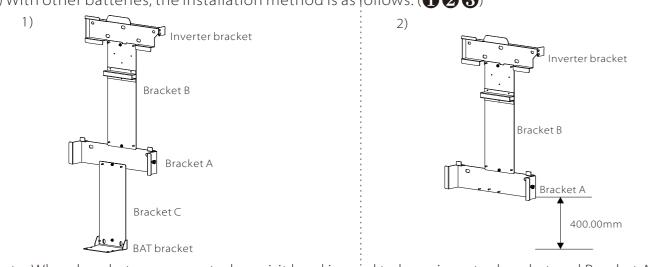
Note: When brackets are mounted, a spirit level is used to keep inverter bracket and Bracket A parallel to the ground.
