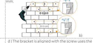
c) Insert expansion bolt into the nine hole, use rubber hammer to knock the expansion screw bolt into the wall.
