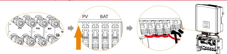
\*\*Note: 5.0 kw and 6.0 kw M series inverter have only two MPPT and two PV strings, so when connecting, you need to unplug ①/② of the PV in the X3-Matebox basic.
