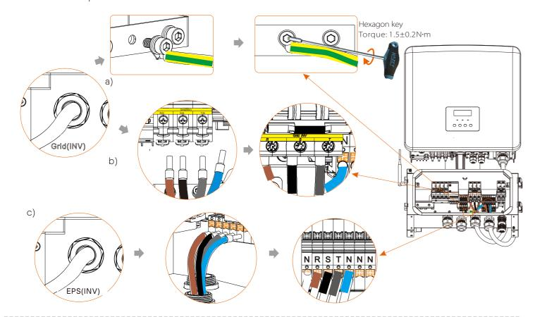
2) Grid (L1/L2/L3/N/PE) /Load (L1/L2/L3/N) side connection
