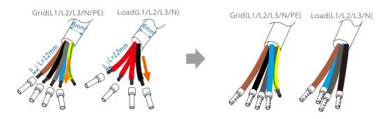
b) Grid (PE) strip the grounding cable, remove the 13 mm insulation layer from the end of the wire. Insert the stripped cable into the R type terminal, and then clamp it.
