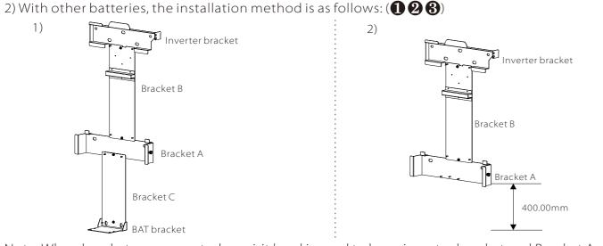
Note: When brackets are mounted, a spirit level is used to keep inverter bracket and Bracket A
