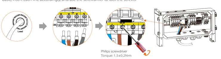
4) Pass the Grid line through the Grid port of the X3-MateBox basic, and then find Grid (N/R/S/T) port inside the X3-Matebox basic. Force the cable harness directly into the hole to jam, gently twist not to loosen. Grid (PE) is locked with a Hexagon key.
