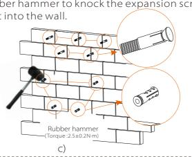
inner hexagonal wrench to screw the tapping screw until the expansion bolt "bang" is heard.
