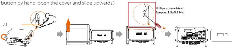
b) Put the matebox on the bracket. Make sure the box is well fixed on the bracket by screwing all nuts
