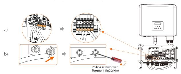
2) Grid(L/N/PE) /Load(L/N) side connection.
