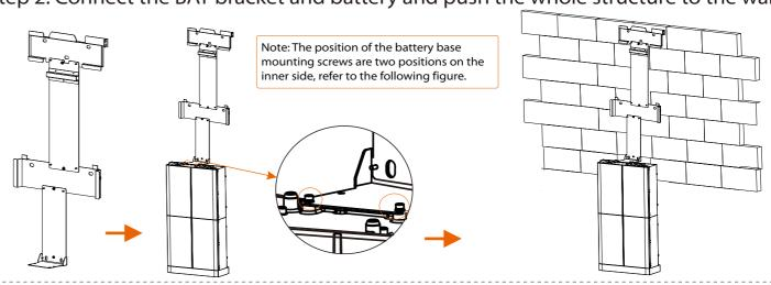
Step 3: Fix the position, drill holes and install the whole structure on the wall
