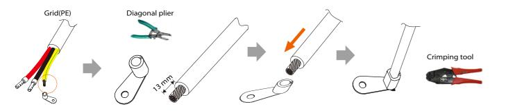
c) Pass the Grid/Load line through the Grid/Load port of the matebox, then find the Grid (L/N) and Load (L/N) ports in the matebox, insert each line accordingly, and use the screwdriver to lock the screws. Grid (PE) is secured with a philips screwdriver.
