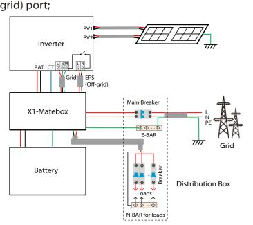
Diagram A: Neutral line and PE line are separated : Diagram B: Neutral line and PE line are combined together, all loads connect to the EPS (Off-grid) port.
